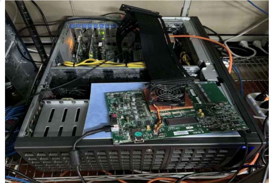
Same host used for OAI optimization and PCIe-connected FPGA offload
