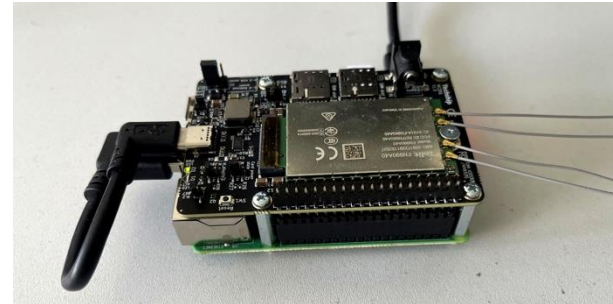
Raspberry Pi-based UE with Telit Modem for SIB-9 Testing
