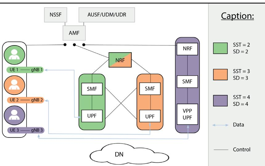
A Network Slice is defined within a Public Land Mobile Network (PLMN), and it incorporates the 5G Core and 5G RAN components. Network slice is identified by a Single Network Slice Selection Assistance Information (S-NSSAI) that consists of a Slice/Service type (SST) and a Slice Differentiator (SD). OAI CN plans to fully support Network Slicing-related procedures according to the 3GPP standards.
