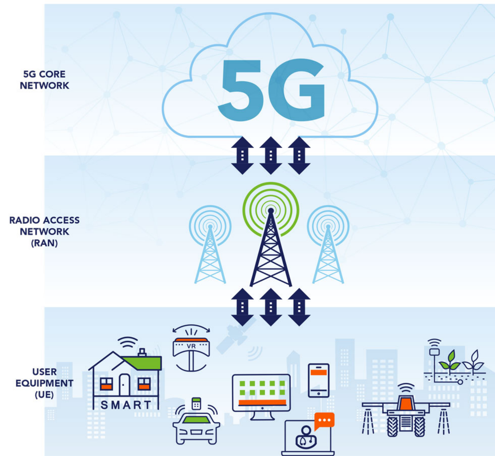
Fig. 1. End-to-End Overview of 5G Networks Architecture [1].
